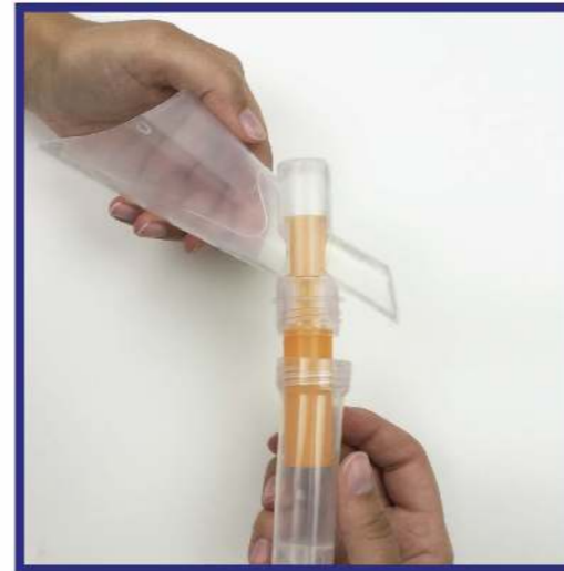
Step 3: Firmly screw funnel onto tube (keep tube upright to prevent spilling the liquid preservative).
